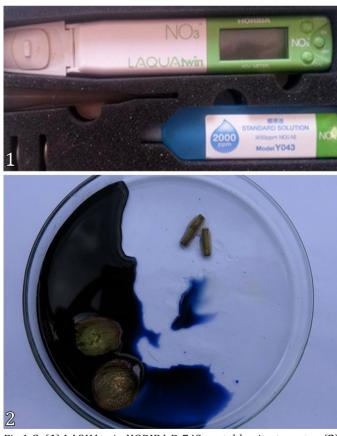
Fig.1-2. (1) LAQUAtwin HORIBA B-743 portable nitrate meter. (2) Diphenylamine test with positive reaction.
